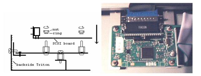
NOTE: If you also have the MOSS-Board installed, take care that the metal tracks do not touch the MOSS-Board. We recommend to put some isolation tape or some carton between the SCSI-Card and the MOSS Board.
