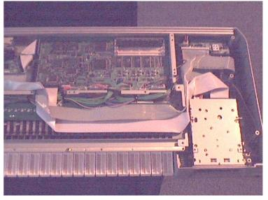
When you mount the bottom be careful that the flat cable isn't squeezed between metal.
